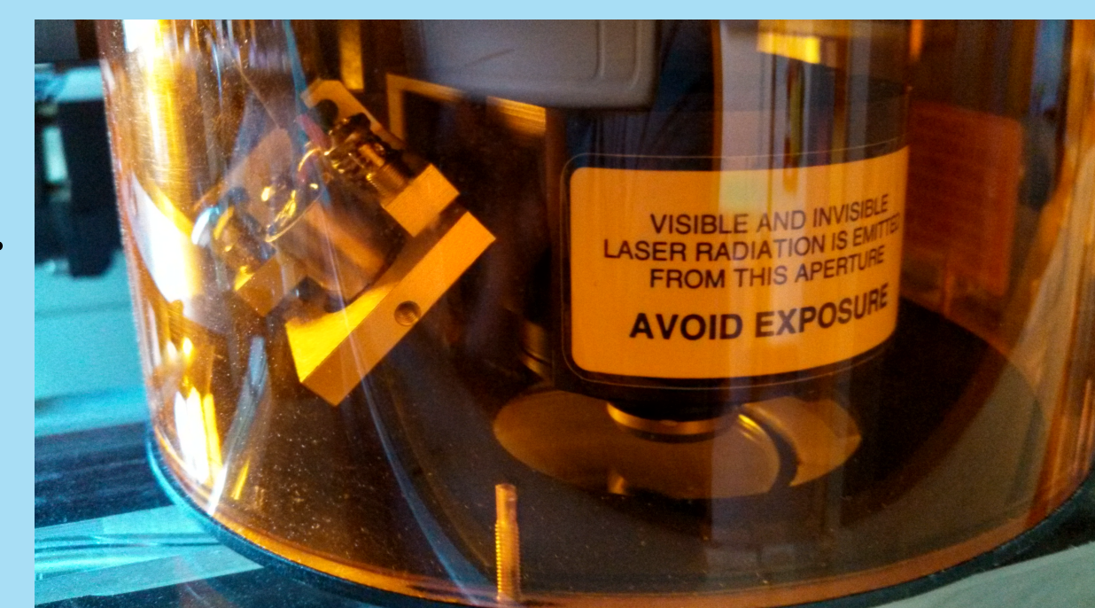
Typical set-up (100 μm beam width, 20 μm resolution) increases the obtainable data points per cm from approximately 1 to 500.
